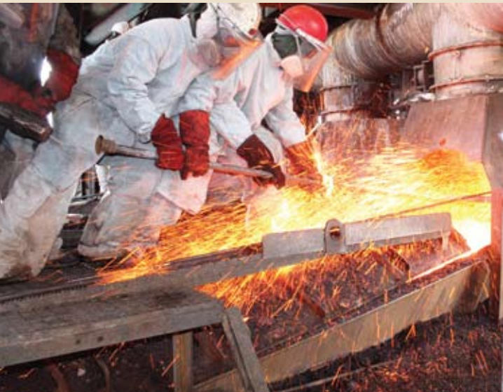
PRECIOUS METAL: Tapping copper matte at the Ausmelt furnace
